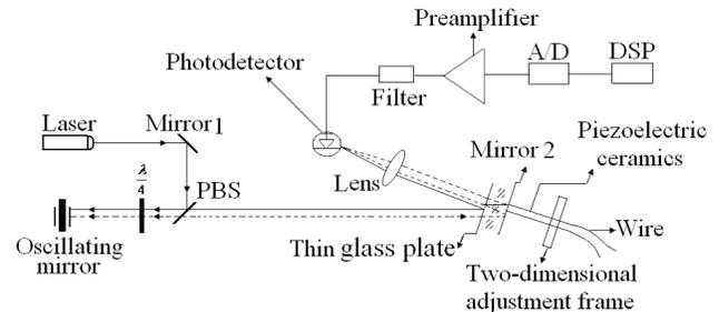
Fig. 3. Scheme of multibeam laser heterodyne measurement electrostriction coefficient.
