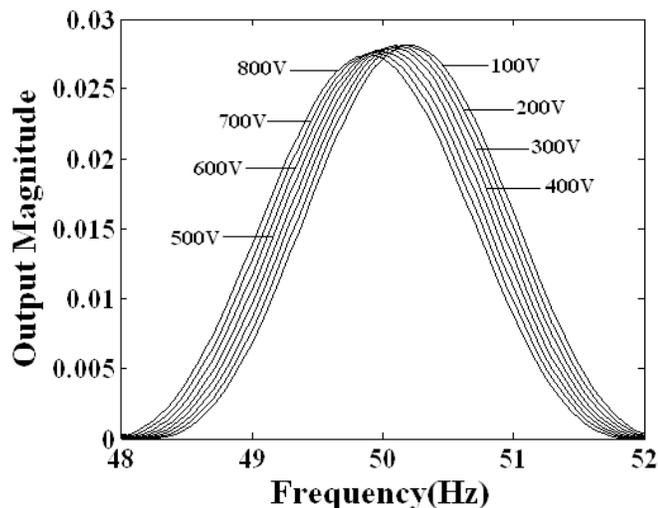
Fig. 5. In the case of different voltages, the spectrum corresponds to the change of PZT length variation.
