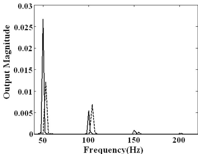
Fig. 4. Fourier transform spectrum of multibeam laser heterodyne signal.
