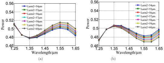
Fig. 4. Wavelength response of different larm<sub>2</sub>: (a) output channel 1 and (b) output channel 2.
