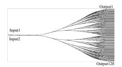
Fig. 6.  $2 \times 128$  optical power splitter.
