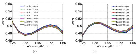
Fig. 5. Wavelength response of different  $larm_1$ : (a) output channel 1 and (b) output channel 2.
