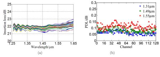
Fig. 8. Performances of 1  $\times$  128 optical power splitter: (a) insertion loss and (b) PDL.
