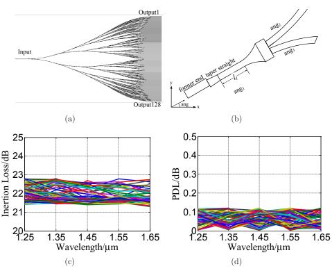
Fig. 1.  $1 \times 128$  optical power splitter: (a) structure, (b) tilt Y-branch, (c) insertion loss, and (d) PDL.
