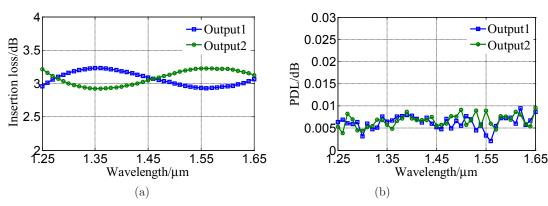
Fig. 6. Simulated results of WINC: (a) insertion loss and (b) PDL.
