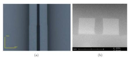
Fig. 7. Photographs of  $2 \times 128$  optical power splitter: (a) micro-photograph after ICP and (b) SEM after top cladding layer.
