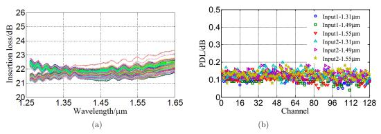
Fig. 9. Optical performances of  $2 \times 128$  optical power splitter: (a) insertion loss and (b) PDL.
