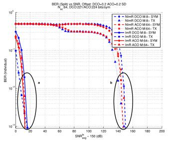
Fig. 4. Comparison of individual BER versus SNR for (a) ImR and (b) NImR.
