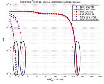
BER vs SNR, N :64, Offset SISO DCO:3.2/ACO:0.0 SD, SIS DCO:3.2/ACO:0.2 SD
