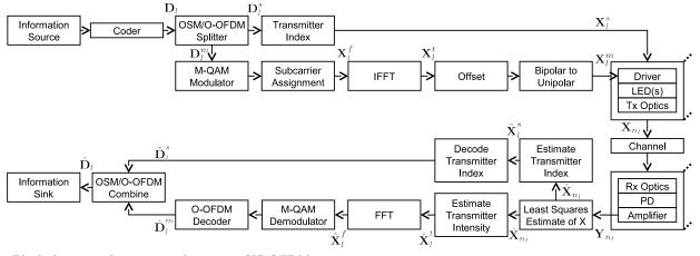
Fig. 1. Block diagram of system implementing SIS-OFDM.
