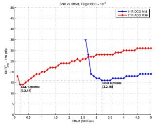
Fig. 2. SNR versus offset for target  $BER = 10^{-3}$  using an ImR.
