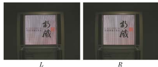
Fig. 9. Viewed images at a left eye position and at a right eye position. Note that there is a binocular disparity between the Chinese characters and the seal.
