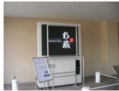
Fig. 8. Developed stereoscopic display by use of 4-mm pitch LED panel.
