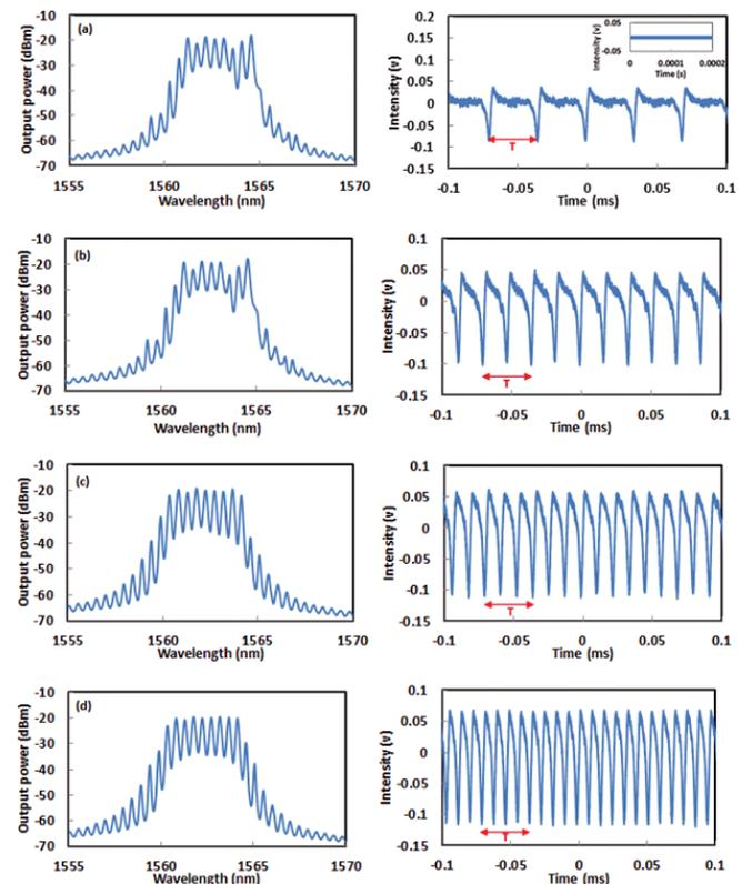
Fig. 3. Optical spectrum and typical mode-locked pulse train of the proposed multiwavelength mode-locked EDFL at four different orientations of PC when the pump is fixed at 146 mW: (a) fundamental, (b) second-order, (c) third-order, and (d) fourth-order harmonic mode locking. Inset of Fig. 3(a) shows the amplitude level of CW laser.
