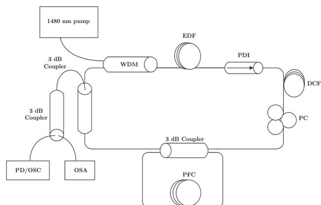
Fig. 1. Schematic diagram of the proposed multiwavelength mode-locked EDFL with a dark pulse emission.
