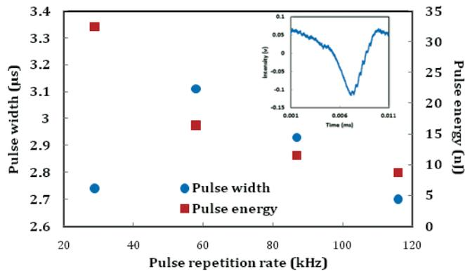
Fig. 4. Pulse width and pulse energy at different orders of harmonic. Inset shows a single dark pulse at fourth-order harmonic.
