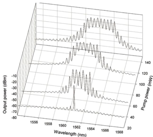
Fig. 2. Multiwavelength output spectrum evolution against 1480 nm pump power.
