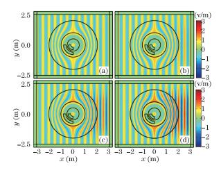
Fig. 7. (Color online) Electric field distribution of a curved sheet covered by the proposed optical device with loss tangents of (a) 0.001, (b) 0.005, (c) 0.01, and (d) 0.015.
