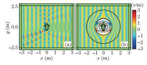
Fig. 5. (Color online) (a) Scattering pattern of a woman-like rigid scatterer. (b) The scatterer in (a) is cloaked by the proposed optical device.
