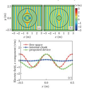
Fig. 4. (Color online) Electric field distribution in the vicinity of (a) the proposed optical device and (b) a traditional internal cloak under plane wave irradiation. (c) Comparison of electric field distributions along the x-axis of the hidden area.
