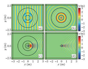
Fig. 2. (Color online) Electric field distribution in the vicinity of the proposed optical device (a) when a plane wave propagates from left to right and (b) when a line source is located at the origin. Electric field distribution of the horn antenna (c) with and (d) without an optical device.
