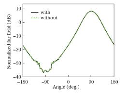
Fig. 3. (Color online) Normalized far field distribution of the horn antenna with and without an optical device.
