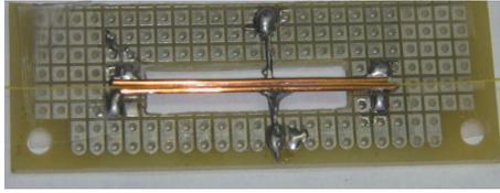
Fig. 1. Optical fiber humidity sensor.
