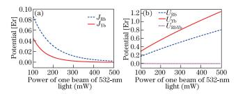
Fig. 3. (a) Tunneling energies of Rb and Yb atoms depend on the power of the 532-nm laser; (b) intra- and interspecies interaction energies of Rb and Yb atoms depend on the power of the 532-nm laser. The interspecies interaction are far smaller than the tunneling and intraspecies interaction when the power lager than 50 mW.
