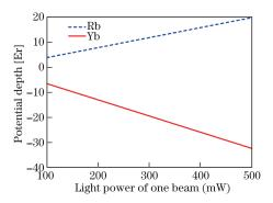
Fig. 2. Potential depth of both species varying with the power of 532-nm laser. Since the Rb and Yb atoms experience reddetuned and blue-detuned lattice potentials, respectively, the signs of their depths are opposite.
