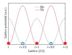
Fig. 1. Light potentials for Rb and Yb atoms in a staggered lattice. The solid and hollow balls depict the Rb and Yb atoms, respectively. The dash and solid lines represent the potential experienced by Rb and Yb atoms, respectively. They are staggered with a spatial separation of 133 nm.
