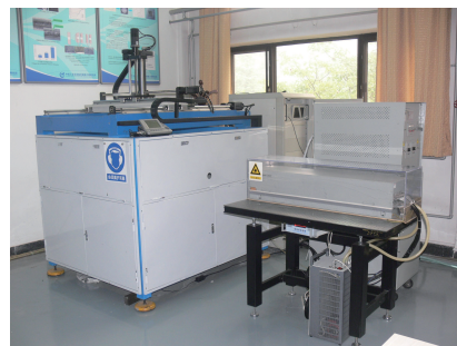
Fig. 1. Setup for laser shock processing in BAMTRI.
