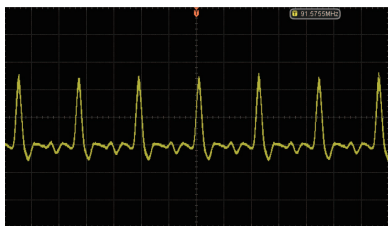
Fig. 3. Temporal behavior of the 1064-nm ps pulsed seed source.
