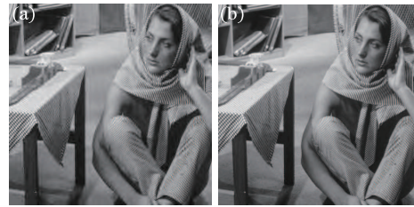
Fig. 5. Decoding results of Barbara using EOCS algorithm based on (6, 14). (a) 0.25 bpp and (b) 1.0 bpp.
