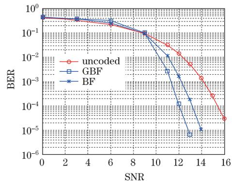
Fig. 3. BER versus SNR values for 4-PPM signals.
