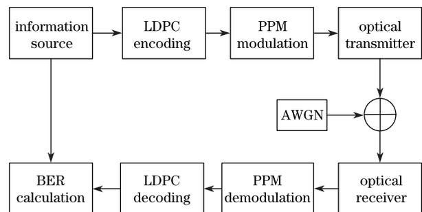
Fig. 1. Block scheme of LDPC coded FSO transmission.
