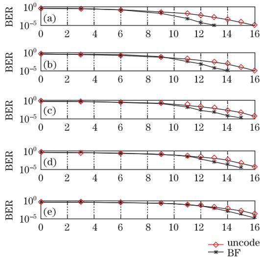
Fig. 2. BER curves versus SNR with PPM modulation numbers of (a) 2, (b) 4, (c) 8, (d) 16, and (e) 64.
