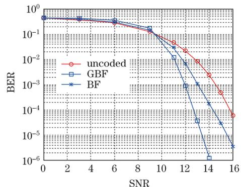
Fig. 4. BER versus SNR values for 16-PPM signals.
