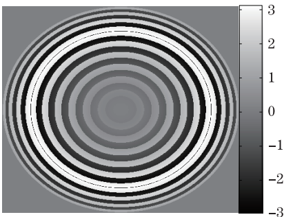
Fig. 3. Pure phase apodizer. The number of phase modulation belts is 20, and the width of the belts is so chosen that the converging semi angle difference of two corresponding radii of each belt is equal with each other.
