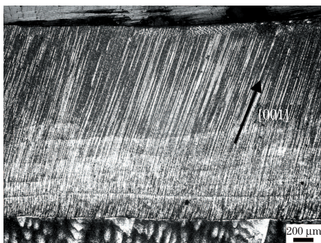
Fig. 8. Cross-section of the solidification microstructure of the laser multilayer-deposited Rene88DT on the DD3 single crystal obtained at \omega=\pi/6 .
