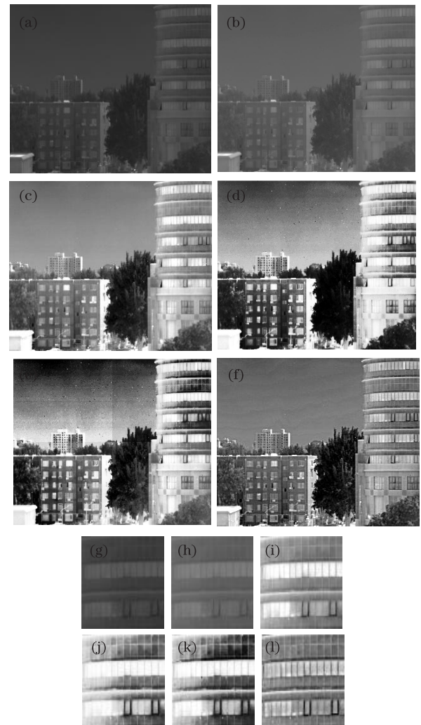
Fig. 5. Experimental results of the sky-terrain scene. (a) Original image; (b) \gamma correction ( \gamma=0.7 ); (c) AGC; (d) GHE; (e) POSHE; (f) LAGC-HSS; (g)–(l) local regions of (a)–(f).
