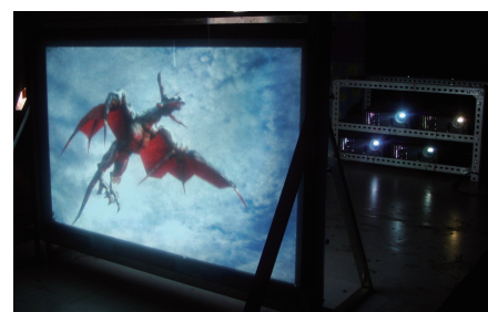
Fig. 4. 50-inch autostereoscopic 3D projection display prototype.
