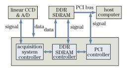
Fig. 1. System block diagram of high-speed spectrum acquisition.
