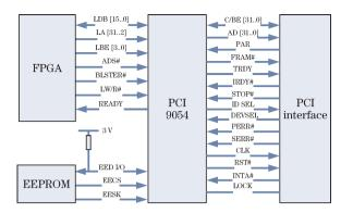
Fig. 6. PCI peripheral interface circuit.
