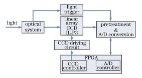
Fig. 2. Functional diagram of spectral acquisition.
