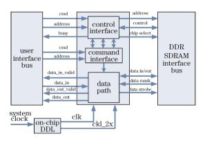
Fig. 5. Internal control modules of DDR SDRAM.
