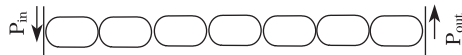
Fig. 3. Schematic of seven coupled micro-ring resonators with two coupled line waveguides as input and output ports.
