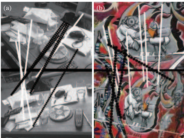
Fig. 1. Illustration of mismatched points resulting from local texture similarity. (a) A photo of a cluttered coffee table; (b) a mural painting. The solid lines represent the correct matches while the dotted lines represent the incorrect ones.
