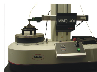
Fig. 3. Industrial form measurement machine with an integrated fiber optical measurement system.
