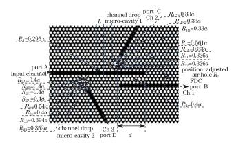
Fig. 1. Structure of the proposed triplexer. The radius of the PC air holes is r = 0.33a, where a is the lattice constant. In the bus waveguide section between the two micro-cavities, the waveguide propagation constant is changed to meet the phase term, and the radius of border air holes in the waveguide section is  $R_3 = 0.295a$ .
