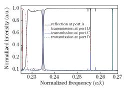
Fig. 4. Frequency response of the triplexer at s = 0.15a calculated using the FDTD method.
