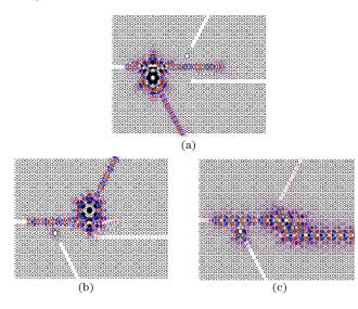
Fig. 3. Steady-state electric field distributions of optical triplexer for the three wavelength signals of (a) 1310 nm, (b) 1490 nm, and (c) 1550 nm.
