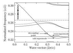
Fig. 2. Dispersion curves for the two-waveguide modes of the FDC. The operational frequencies of the triplexer are denoted by the solid, dashed, and dot-dashed lines, and the normalized frequencies are  $0.22614(a/\lambda)$ ,  $0.23525(a/\lambda)$ , and  $0.26757(a/\lambda)$ , respectively, whose corresponding wavelengths are 1550, 1490, and 1310 nm, respectively, for the lattice constant of 350.5 nm. The inset shows the supercell of the calculated W1 PC waveguide (W1 means one row of holes).
