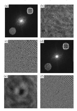
Fig. 3. Experimental results using the cervical cancer cell TZMbl as sample: (a)–(c) with the existence of the object, the reconstructed amplitude image of the whole field, part of the real image in the pane of Fig. 3(a), and the wrapped phase image, respectively; (d)–(f) with the absence of the object, the reconstructed amplitude image of the whole field, part of the real image in the pane of Fig. 3(d), and the wrapped phase image.
