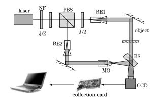
Fig. 1. Schematic diagram of LFTDH configuration. NF: neutral filter. BE: beam expender; MO: microscope objective.
