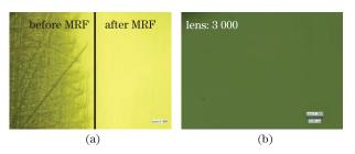
Fig. 3. KDP surface appearances after polishing. (a) Comparison of surface before and after MRF and (b) KDP surface micro-shape after MRF.
