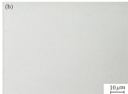
Fig. 5. Photomicrograph of polishing (a) without the surface modification cladding, (b) after coating the surface modification cladding.
