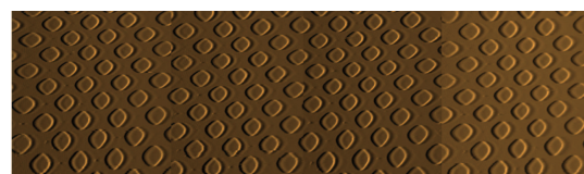
Fig. 6. The large-range image of 2D grids formed by splicing four sequential images together. The total size is 68 \mu\text{m} .
