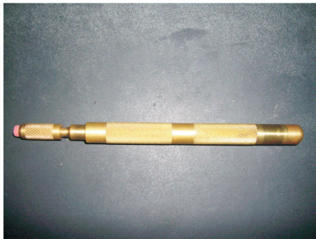
Fig. 1. Copper pen with rubber eraser for testing abrasion resistance.
