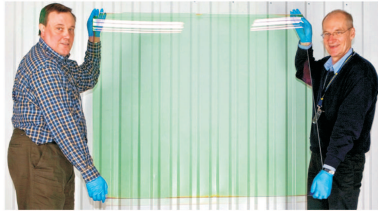
Fig. 9. 1.2 \times 1.2 (m) substrate for PV application, coated by an in-line ALD tool.
