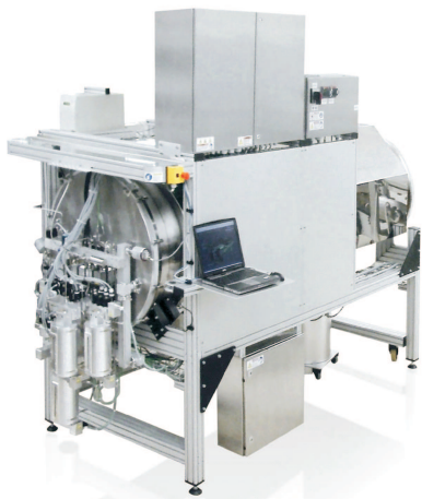
Fig. 10. Example of an industrial ALD batch coater for optical films [9] .
