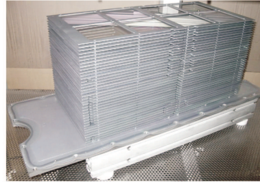
Fig. 4. Example of the \text{TiO}_2 batch for uniform ( \pm 2\% ) coatings, 36 shelves 240 \times 500 (mm), double-sided coatings ( 8 \text{ m}^2 of a film).
