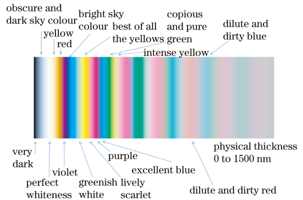
Fig. 4. Fringes that Newton observed in a soap bubble and the names he identified for each. In fact, Newton recorded fringes out of that labeled "dilute and dirty blue" (Courtesy of Thin Film Center, Inc.).
