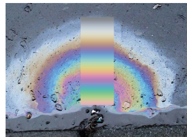
Fig. 5. Photograph of diesel spill on a road (from Wikimedia Commons, taken by user Guinnog). Superimposed on the photograph is a color strip exhibiting the results of calculating the color of fringes in an oil film over water. The film is linearly wedged from zero thickness (top) to 500 nm physical thickness (foot). The D_{65} illuminant and the 1931 CIE observer were employed in the color calculation. Color calculation courtesy of Thin Film Center Inc. (This composite illustration is freely available under the terms of the Wikimedia Commons license).
