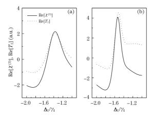
Fig. 4. Variation of  $\operatorname{Re}[\chi^{(3)}]$  (solid curves) and  $\operatorname{Re}[T_1]$  (dotted curves) versus the probe detuning  $\Delta_1$  with  $\Omega_3 = \gamma_4$ . (a)  $\Omega_2 = 0.5\gamma_4$ , (b)  $\Omega_2 = 1.0\gamma_4$ . Other parameters are the same as those in Fig. 2.
