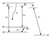
Fig. 1. Schematic diagram of the studied system. It consists of three lower levels and a single upper level. The lower states are coupled near-resonantly to the excited state by  $\Omega_1, \Omega_3$ , and  $\Omega_4$ , respectively, and a microwave field is applied to  $|2\rangle \leftrightarrow |3\rangle$ .
