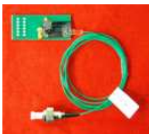
Fig. 3. Unpackaged triplexer chip.
