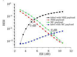
Fig. 4. BER versus ER in FSK/IM system with NRZ and MC payload.
