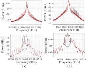
Fig. 3. Spectra of combined FSK/IM signal with NRZ label and (a) NRZ payload, (b) MC payload (resolution bandwidth 0.01 nm).
