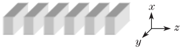
Fig. 1. Schematic of the PBG structure with a double-layer unit cell of an air layer and an anisotropic LHM layer.
