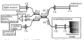
Fig. 1. Schematic of the OCT system. FC: fiber coupler; PC: polarization controller; OL: objective lens; D: detector; CL: collimating lens.
