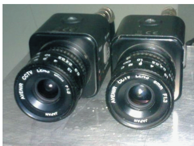
Fig. 3. Setup of the stereo camera for shooting the parallax images.
