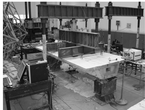
Fig. 3. Strain measurement of the RC box-girder in bending.
