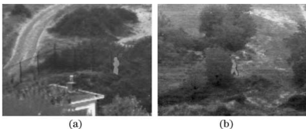
Fig. 1. Two false color images formed by assigning IR image to R channel, LLL image to G channel, and zero value to B channel. The ratio between the IR and LLL sensor outputs approximately reflects the depth relationships for same materials. Regarding the same kind plants, near ones appear redder (higher color saturation) than the distant ones (i.e., the ratio is higher).
