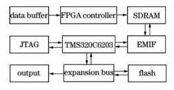
Fig. 4. Hardware configuration of the DSP system. SDRAM: synchronous dynamic random access memory; JTAG: joint test action group; EMIF: external memory interface.
