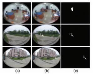
Fig. 6. Detection results of background subtraction method. (a) Backgroud images; (b) images to be detected; (c) detection of the object.
