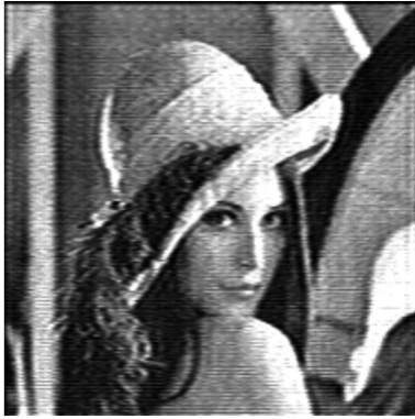
Fig. 6. Reconstruction of the 1-bit, half-toned 'Lenna' image from hologram derived from sub-lines generated with the FIR filter setting in Table 2.
