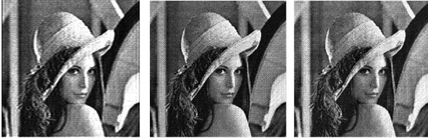
Fig. 5. (a) The half-toned ‘Lenna’ image; (b) reconstruction of a hologram representing (a). The hologram is derived from sub-lines generated with 8-bit filter coefficients based on the optical setting in Table 1, followed by applying Eq. (2). (c) Reconstruction of a hologram representing (a). The hologram is derived from sub-lines generated with 1-bit filter coefficients based on the optical setting in Table 1, followed by applying Eq. (2).
