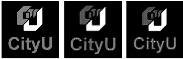
Fig. 7. (a) A half-toned image containing a logo (upper half of the image) and a text message (lower half of the image) located at 51.5 and 48.5 cm from the hologram, respectively. (b) Reconstruction of the hologram, generated with the proposed method, representing the half-toned image in (a). The reconstruction distance is 48.5 cm. (c) Reconstruction of the hologram, generated with the proposed method, representing the half-toned image in (a). The reconstruction distance is 51.5 cm.
