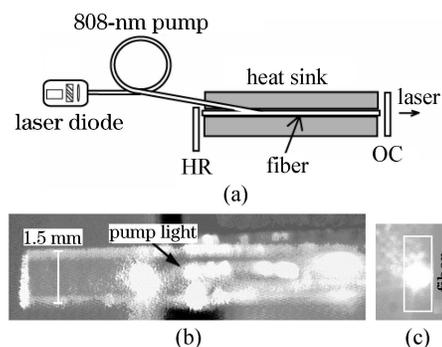
Fig. 1. (a) Schematic of experimental setup. HR: high reflective mirror, OC: output coupler; (b) top view and (c) side view of pump light trace inside the fiber. The white rectangle indicates the region of the fiber core.
