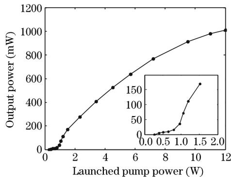
Fig. 2. Output power versus launched pump power. Inset: output power near threshold.
