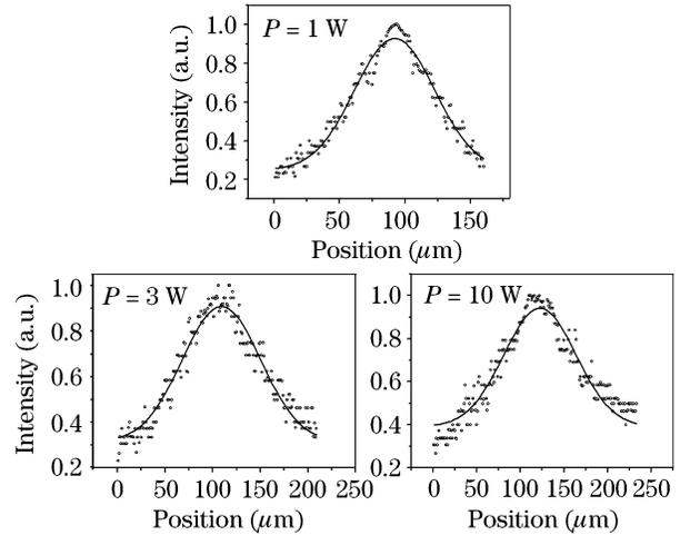
Fig. 3. Near-field laser beam profiles for various pump powers. Solid curves are Gaussian fits to the measured data.
