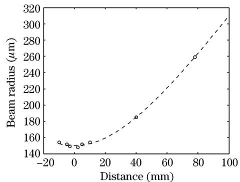
Fig. 4. Beam width as a function of propagation distance. Dashed line is calculated with  $M^2 = 1.2$ .
