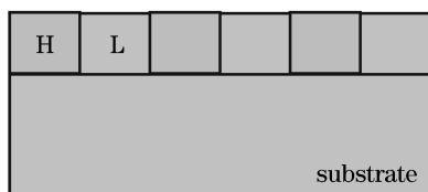
Fig. 1. Structure of single-layer GMRF. n_{gH} = 2.35 , n_{gL} = 1.46 , n_{sub} = 1.46 , \Lambda = 400 nm, f = 0.5 .
