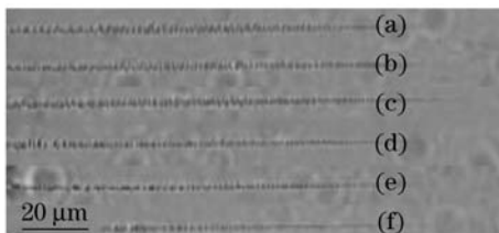
Fig. 6. Void array induced at the focal depth of 150 \mu m with the entrance surface of the laser beam parallel to the (010) crystal plane.
