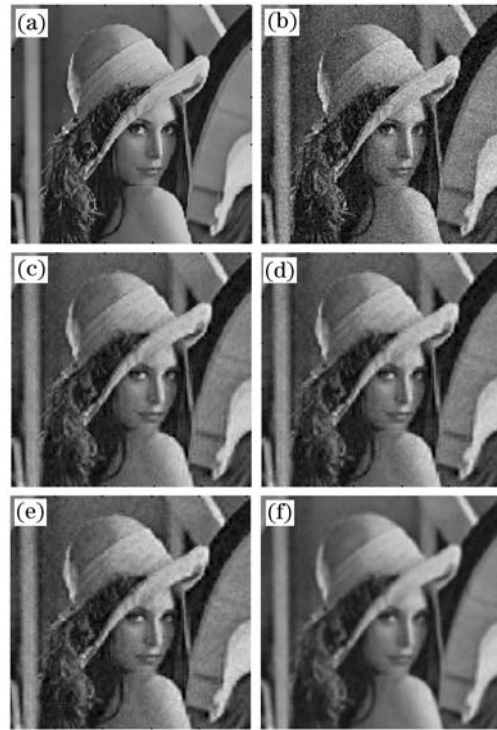
Fig. 2. Comparison of different denoising methods for Lena image with PSNR = 24.04. (a) Original Lena image; (b) noisy Lena image; and denoised images by using (c) the proposed method, (d) Gaussian RBF, (e) polynomial RBF, (f) median filtering.
