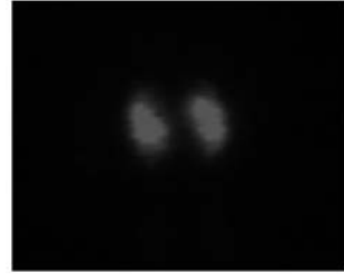
Fig. 6. Near field profile of the output beam with apertures.
