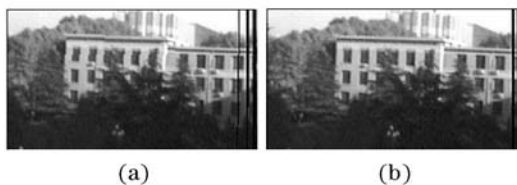
Fig. 3. Illustration of boundary error. (a) Artifacts near the boundary (right) due to error propagation; (b) result of error modification.
