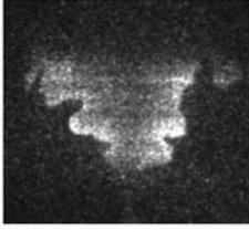
Fig. 2. An OH-PLIF image of a V-flame.
