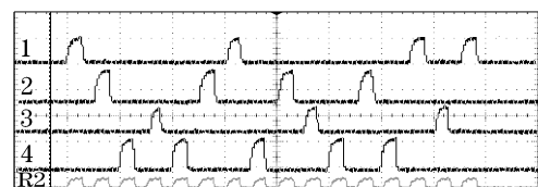
Fig. 3. Outputs of five photodiodes after correlation process with memorial patterns. Channel 1 correlated with Fig. 2(a); channel 2 correlated with Fig. 2(b); channel 3 correlated with Fig. 2(c); channel 4 correlated with Fig. 2(d); channel R2 is the clock signal from laser2.
