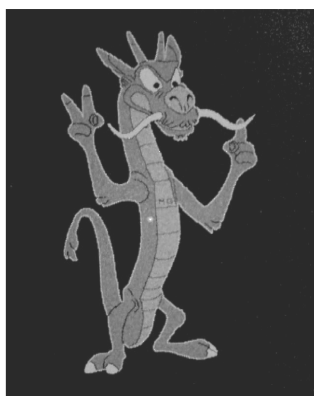
Fig. 1. Output of a computer-generated diffractive optical element calculated by an iterative design algorithm.
