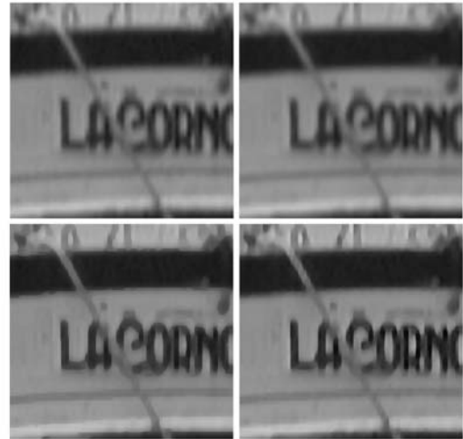
Fig. 5. Enhancement of part of the boats image by different methods: from top-left to bottom-right, noisy blurred image, images enhanced by AD, ADSF and FBDF, respectively.
