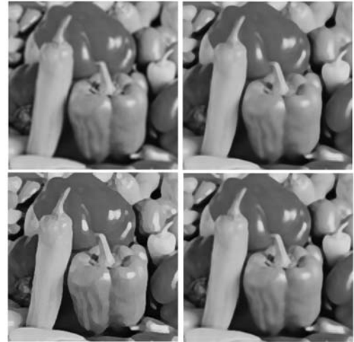
Fig. 4. Enhancement of the peppers image by different methods: from top-left to bottom-right, noisy blurred image, images enhanced by AD, ADSF and FBDF, respectively.
