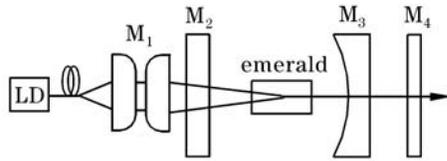
Fig. 3. Experimental setup of emerald laser.
