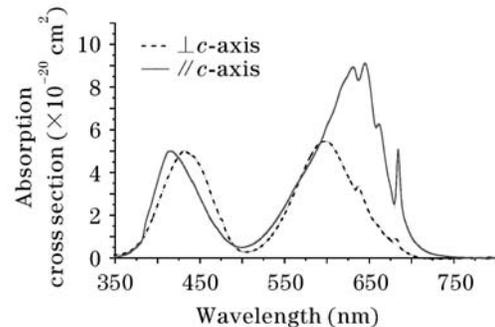
Fig. 1. Polarized absorption spectra of emerald crystal.
