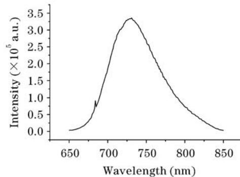
Fig. 2. Fluorescence spectrum of hydrothermal emerald.
