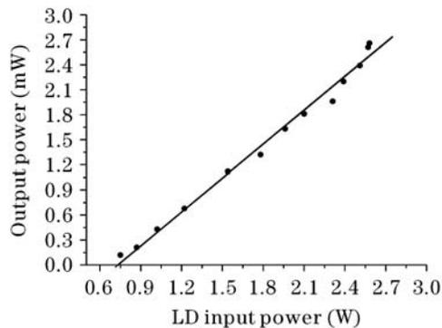
Fig. 4. Output power at 731 nm as a function of LD incident power with the rod length of 10.5 mm.
