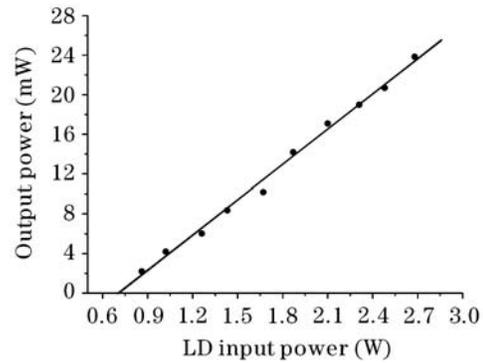
Fig. 5. Output power at 731 nm as a function of LD incident power with the rod length of 3.4 mm.
