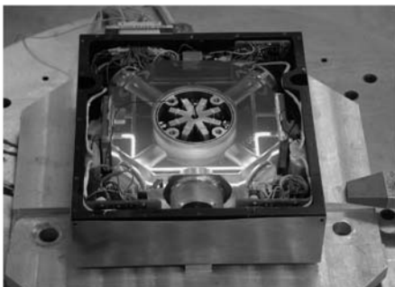
Fig. 1. High-precision single-axis RLG.
